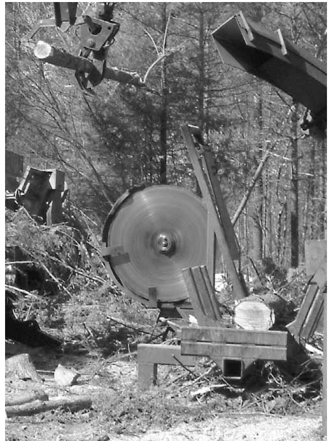
Slasher blades and circular saw firewood processor saws are identical.
