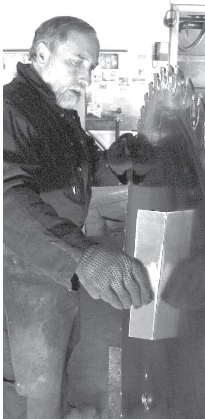
Checking the saw with a 12-inch straightedge.
