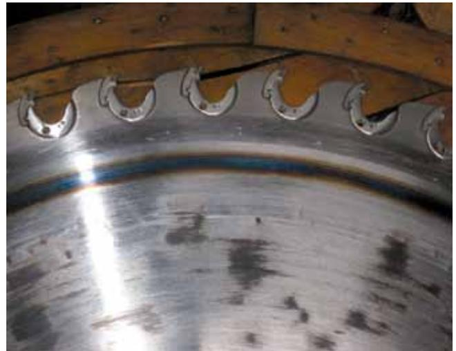
have caused some collar damage. But whatever turned this saw blue didn't happen while the pins were sheared because that would have left the saw standing still while the mandrel continued to rotate.
