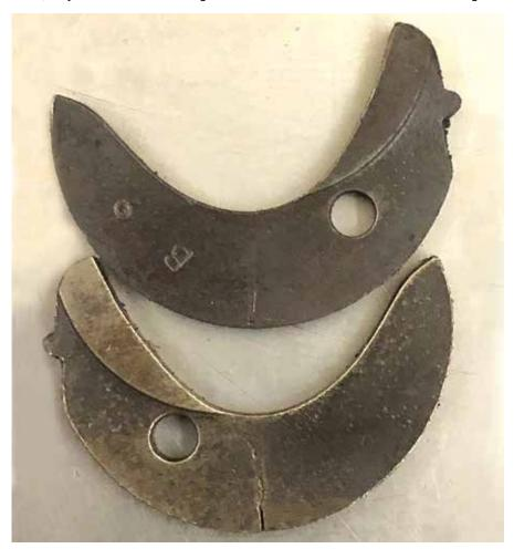
Notice the crack at the bottom of the shank.
