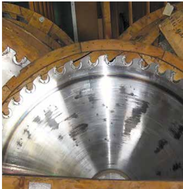
The guideline got very hot (blue) on this saw. The black patches are softwood pitch, showing the clear presence of high and low spots.
