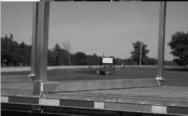
Unique center web design makes the Alum-A-Log Stakes 50% stronger and 50% lighter than most steel stakes. One Crossbar and 2 stakes only weigh 91 lbs.
