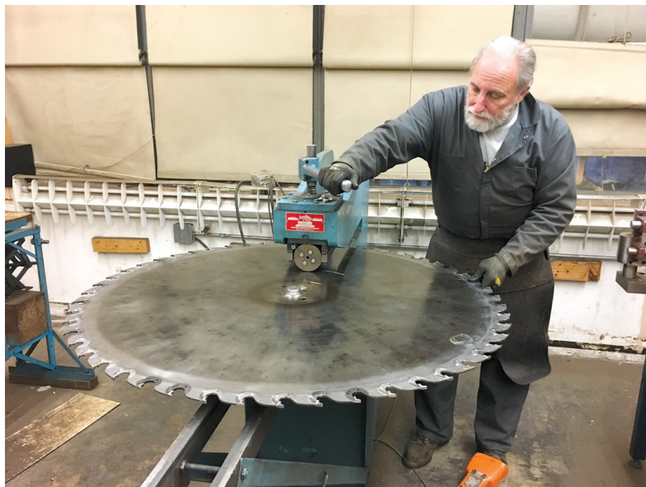
Determining the proper amount of force applied with the stretcher roll is not much different than making the same determination with a hammer.
