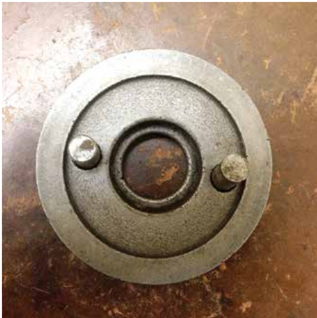
5/8” pin holes with 9/16” pins.
