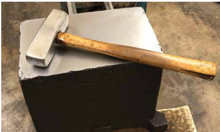
A 4 ½ pound Combination Hammer on a sawmaker's anvil.
